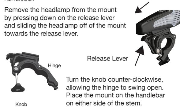
Turn the knob counter-clockwise, allowing the hinge to swing open. Place the mount on the handlebar on either side of the stem.
