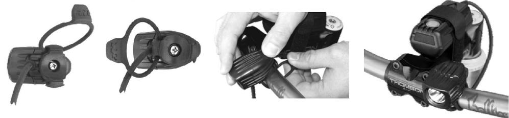
**TIP:** The 2 slots on the mounting assembly are different sizes. The larger slot opening should face the back of the bike, giving more room for attaching the mounting strap. The smaller slot opening should face forward, reducing the chance of dropping the mounting strap.
