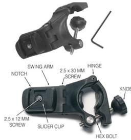
The UHM can be adjusted to accommodate any handlebar angle. By loosening the 2.5 x 30 mm Allen screw, you can move the swing arm back and forth to straighten the headlamp. Tighten the 2.5 x 30 mm screw after the adjustment.
